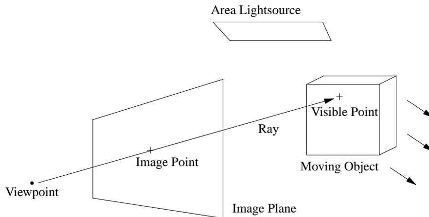
Figure 18. Distributed Ray Tracing
