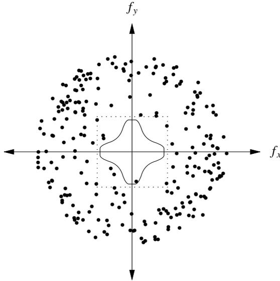
Figure 14. Spectrum of Nonuniformly Sampled Image
