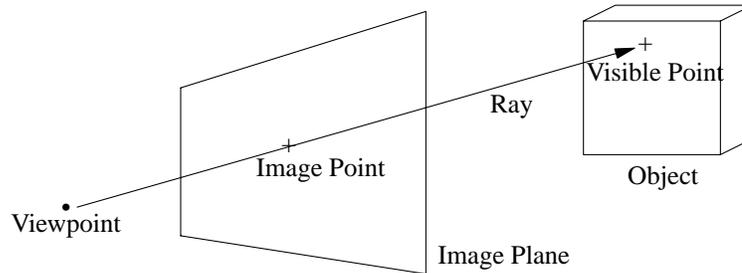
Figure 2. Basic Ray Tracing
