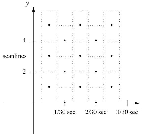
Figure 21. Interlaced Spatiotemporal Box Filter
