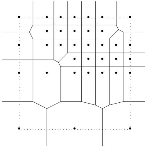
Figure 9 Voronoi Cells of Adaptive-Sample Locations
