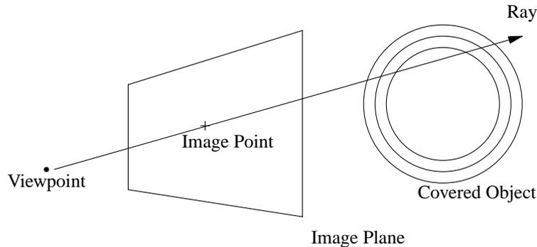
Figure 5. Ray Tracing with Covers
