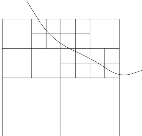
Figure 7. Subdivided Pixel Area in Whitted's Algorithm
