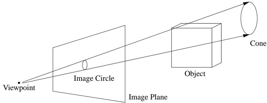
Figure 3. Cone Tracing
